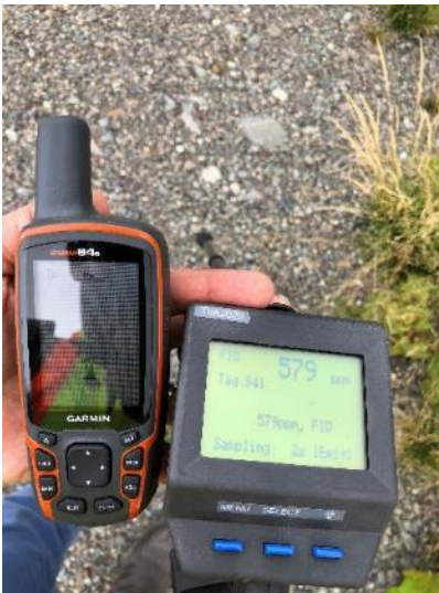
Photos 4 & 5 – Identifying Emission Hotspots during Baseline Emission Surface Scan
