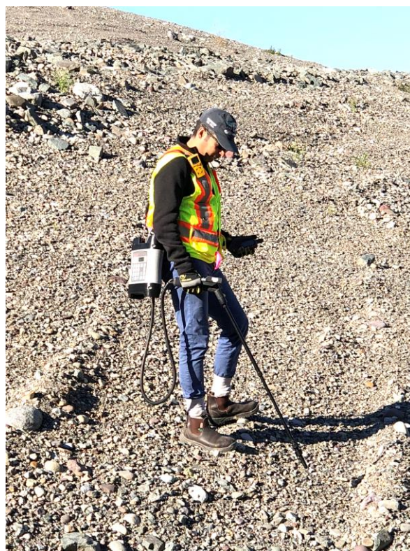
Photo 3 - Surface Methane Concentration Scan Using a Portable FID Instrument
