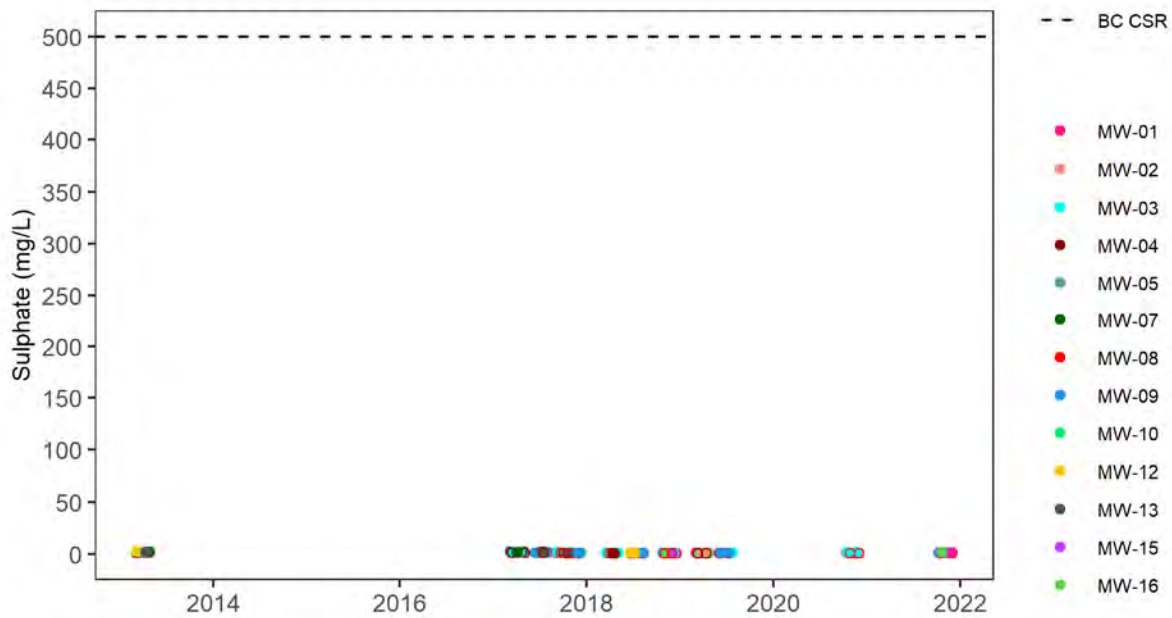
Figure B-9: Temporal plot of sulphate groundwater concentrations, 2013 to 2021.
